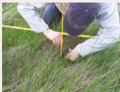
Researchers are collecting field data in Australia and New Zealand by counting the number of live and dead grasses that come into contact with a thin steel rod measuring device, called a Levy Rod, seen at left.
