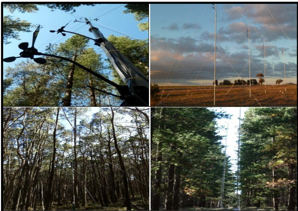
Figure 1. measurement of both horizontal and vertical winds in different vegetation types and open areas at multiple heights
