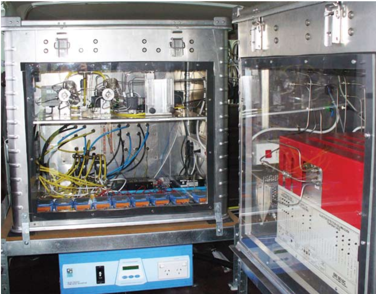
◀ Figure 3: A Gas chromatograph (on the right with red casing, used to analyse N 2 O and CH 4 ) and an InfraRed Gas Analyser (to the left, used to analyse CO 2 ) are housed in the back of the 4WD of the RDGG Lab.
