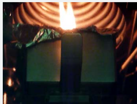
Figure 2: Eucalyptus saligna litter burning inside the mass loss calorimeter
