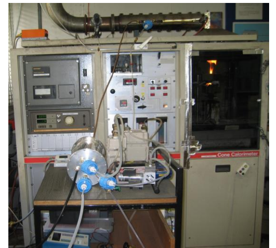
Figure 1. Cone calorimeter experimental setup
