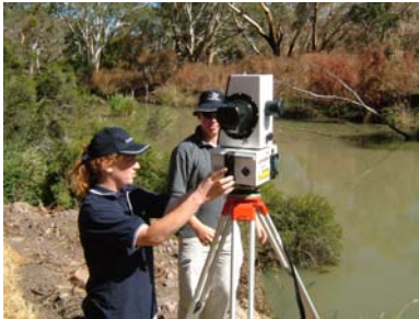
Above: I-SITE 4400LR laser scanner
