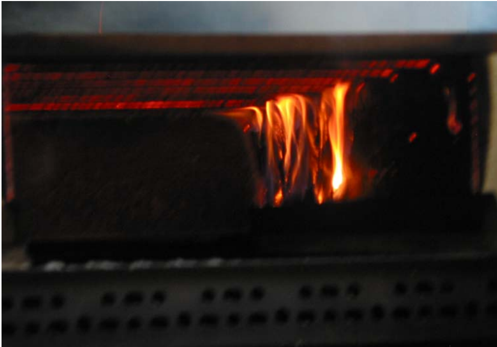
Figure 3-5 Heat from the burning pine joists impinging on the decking
