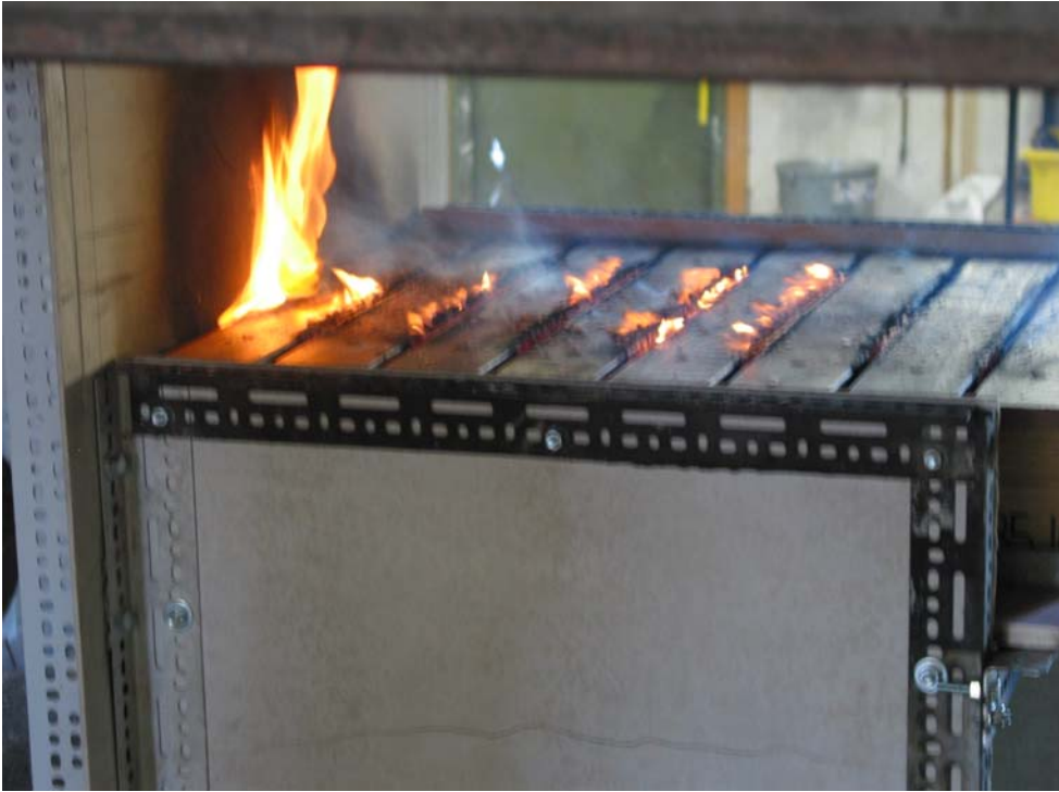
Figure 3-4 Plinth detail causes severe heat load on adjacent wall
