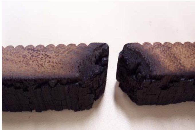
Figure 3-6 Tapered burn pattern on edge of decking boards
