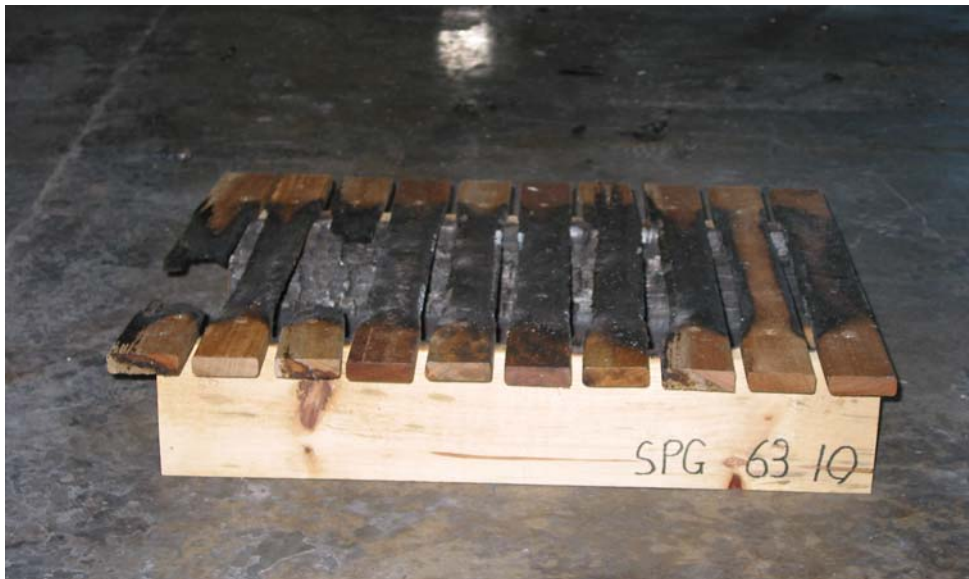
Figure 3-1 A Typical Deck after Testing
