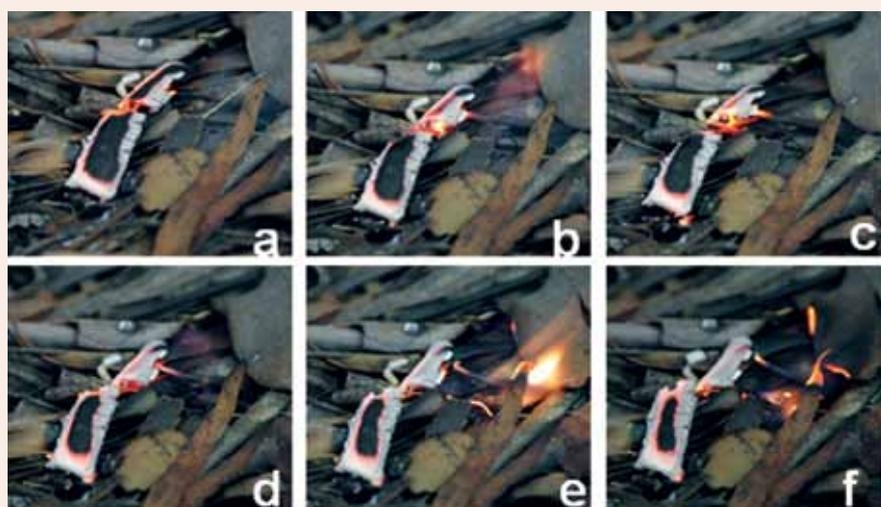
▲ Figure 1: A sequence of six images 0.1 seconds apart showing the ignition of dry eucalypt litter by a glowing firebrand. The firebrand samples were selected to have the combustion and aerodynamic characteristics of small firebrands from the dry forests of southern Australia. See the 'Fire initiation from firebrands' section on page 2.
