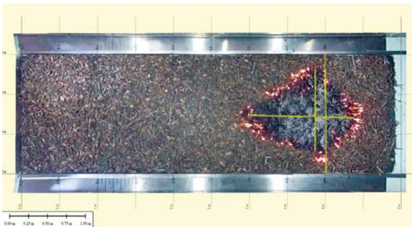
▲ Figure 4: Rectified plan image of an experimental fire in the CSIRO Pyrotron. From a series of such images, rate of spread can be measured with great precision.
