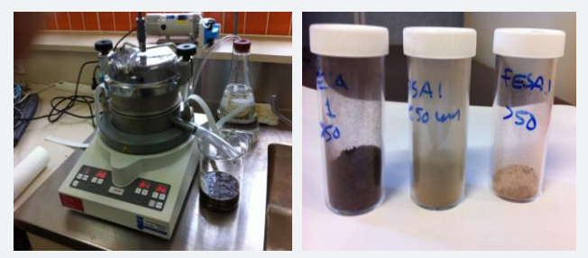
Automated wet-sieving shaker and soil fractions after sieving (50 µm)
