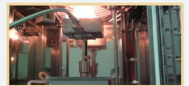
Fuel burning in mass-loss cone calorimeter
