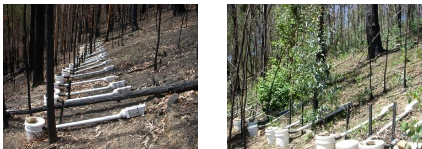
Figure 5: Transect of 20 runoff samplers on the high severity hillslope. Samplers were located 100 m from the ridge on planar hillslopes. The total length of the hillslopes was approximately 200-300 m.
